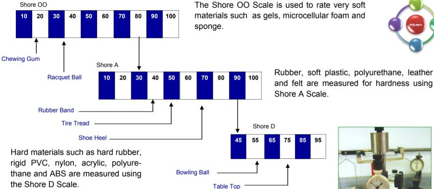
Durometer is the International Standard for measuring the hardness of rubber, sponge, plastic and other non-metallic materials.
